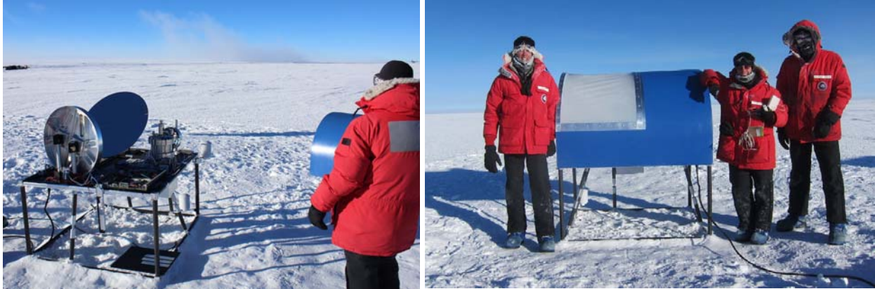
Figure 2: (left) The 3-mirror off-axis Gregorian telescope, cryogenic receiver system and frozen PI are visible in this image. (right) Enclosed in a fiberglass shell and teflon film “window” that is transparent to THz radiation, the HEAT telescope is ready for observations (January 2014).
