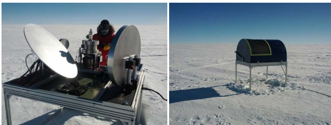
Figure 2: (left) The prototype 3-mirror off-axis Gregorian telescope, cryogenic receiver system and frozen PI are visible in this image. (right) Enclosed in a fiberglass shell and thin black HDPE “window” that is transparent to THz radiation, the HEAT telescope is ready for observations (January 2012).
