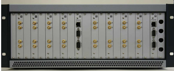
Figure 16: The assembled 8-board, 16 GHz FFT spectrometer from Co-PI Walker's SuperCam-1 project is no larger than a rack-mounted PC and requires only 200 watts of input power. One additional spectrometer module will be purchased for ASTRO.
