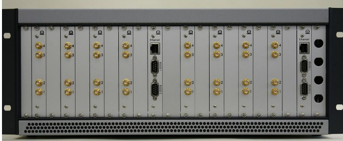
Figure 9: The assembled 8-board, 16 GHz FFT spectrometer from the PI's Supercam project is no larger than a rack-mounted PC and requires only 200 watts of input power! One-fourth of this spectrometer system will be purchased for HEAT.
