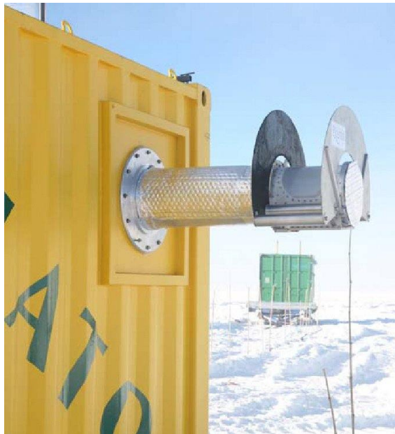
Figure 1: The Pre-HEAT telescope, installed at Dome A with the PLATeau Observatory (PLATO). A technological prototype for the proposed HEAT telescope, Pre-HEAT has a 20 cm clear aperture combined with a 660 GHz Schottky diode receiver and a digital FFT spectrometer. It was deployed to Dome A on an overland traverse led by the Polar Research Institute of China. Its measurements of the submillimeter opacity at Dome A are the basis for the expected performance of HEAT described in this proposal. Preliminary astronomical observations have been performed and the first astronomical spectra are being processed.
