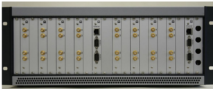
Figure 6: The assembled 8-board, 16 GHz FFT spectrometer from the PI's Supercam project is no larger than a rack-mounted PC and requires only 200 watts of input power! One-fourth of this spectrometer system will be purchased for HEAT.
