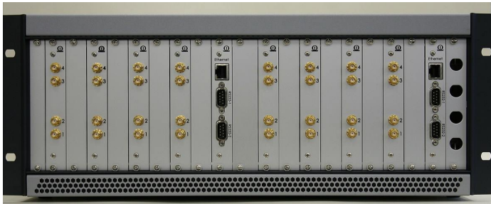
Figure 10: The assembled 8-board, 16 GHz FFT spectrometer from the PI's Supercam project is no larger than a rack-mounted PC and requires only 200 watts of input power! One-fourth of this spectrometer system will be purchased for HEAT.
