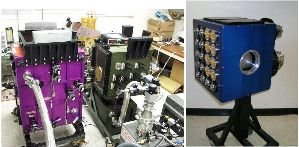
Figure 7: [LEFT] The purple imager and green spectrometer halves of the Arizona Infrared Imager and Echelle Spectrometer, slated for first light at the adaptive optics focus of the 6.5-meter MMT in December 2006. [RIGHT] Supercam, a 64-beam heterodyne receiver operating in the 345 GHz atmospheric window, slated for the HHT. Both instruments are unique and dovetail into the proposed science program.
