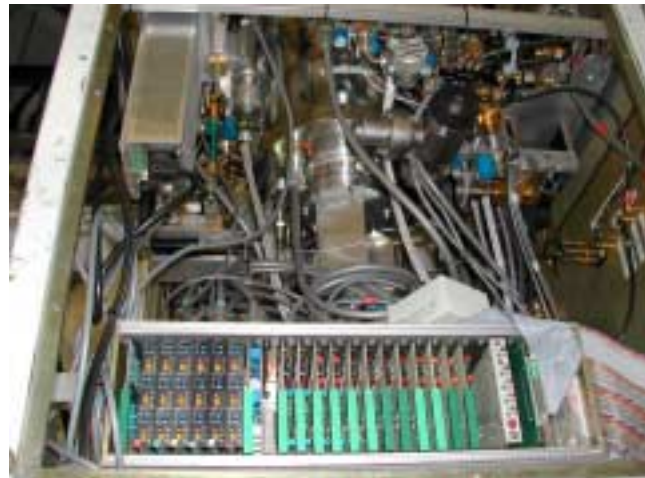
Figure 22: The complexity of the existing 3mm (shown above) will be greatly simplified both electrically and mechanically with the HEMT upgrade.
