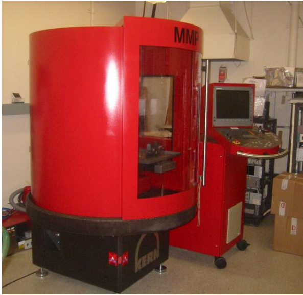
Figure 15: Kern micro-milling machine in the PI's laboratory, used for fabricating devices at frequencies < 1 THz.
