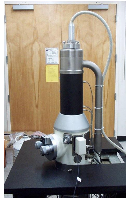
Figure 5: Amray 1000a scanning electron microscope to be used as an electron beam source in initial TWT measurements.
