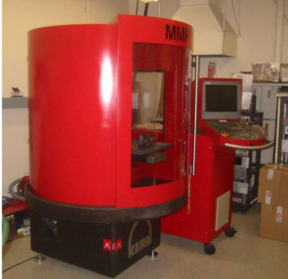
Figure 14: Kern micro-milling machine in the PI's laboratory, used for fabricating devices at frequencies < 1 THz.
