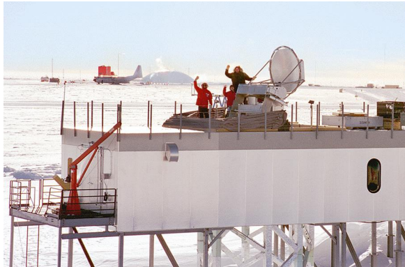
Figure 3: The 1.7-meter Antarctic Submillimeter Telescope and Remote Observatory (AST/RO) has been in continual operation at the Amundsen-Scott South Pole Station since 1994.
