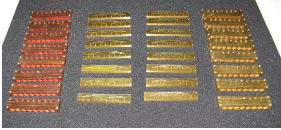
Figure 4: Fully machined extended feed horns for the mixers and LO power dividers, and split-block halves of the corporate 8x8 LO power divider, machined using the Kern micromilling machine purchased largely through this grant.
