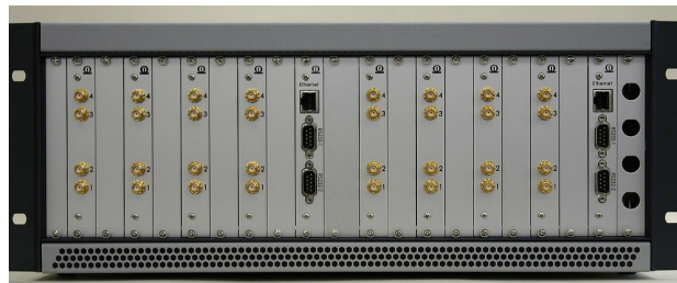
Figure 12: Completed and delivered polyphase filterbank spectrometer system from Omnisys AB. Eight spectrometer cards provide 64 independent receivers with 256 MHz of bandwidth in 1024 channels each, in a single PC-style case with 200 watts of power consumption.
