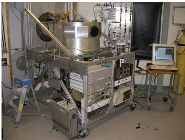
Figure 1: DesertSTAR mounted at the Nasmyth focus of the HHT during its first multipixel engineering run.
