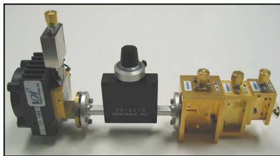
Figure 15: Virginia Diode solid state LO chain.
