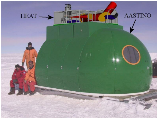
Figure 9: Rendering of HEAT atop a UNSW AASTINO
