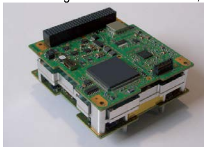
Figure 2. SyrLinks X/S Band Transceiver
