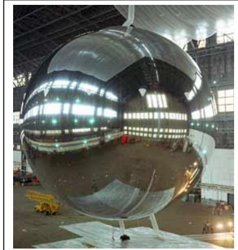
Figure IV.3: Echo 1 Satellite during tests in 1960: 30.5 m in diameter, 0.5 mil Mylar.
