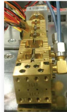
Figure 3. Left: block diagram of the proposed 4-pixel local oscillator unit. It has a single input that accepts power at W-band, a module that divides and amplifies the power into 4 separate channels, a low-frequency module in which the first two stages are housed in the same block, and a block containing the final stage tripler with integrated horns. Right: a 4-pixel 1.9 THz local oscillator under development at JPL.
