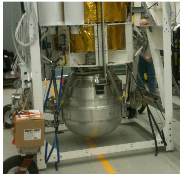
Figure 11: STO Cryostat mounted to telescope (Payload #1, Willy Field, Dec. 2011)
