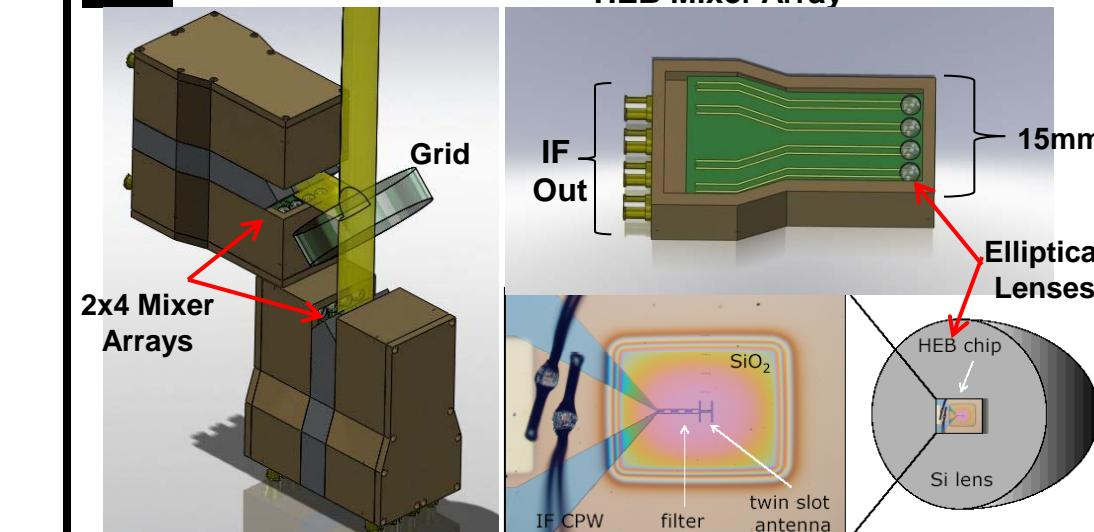
Prototype 500GHz Quasi-optical array- SRON
