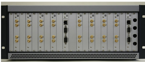
Figure 16: The assembled 16 GHz FFT spectrometer from the PI's Supercam project is no larger than a rack-mounted PC! The equivalent of half of this spectrometer will be purchased for STO.
