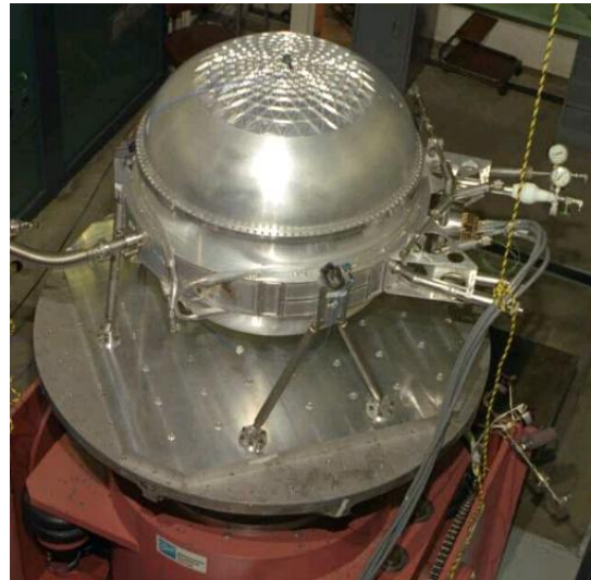
Figure D-11: LLC cryostat during cold vibration tests.
