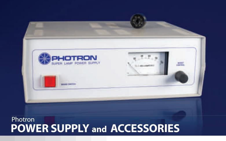
The Photron Super lamp power supply adds a boost discharge for use with Super lamps, the lamp uses existing spectrophotometer lamp current, the power supply adds a boost discharge to increase excitation of atoms sputtered by the instrument lamp supply. This boost current is linked by circuitry inside the power supply and the boost discharge is transmitted at the same rate as the instrument.
