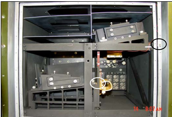
23. Mating Dewar - Temperature sensor # 7 (Outer shield) and # 8 (Inver Frame) are circled above.
