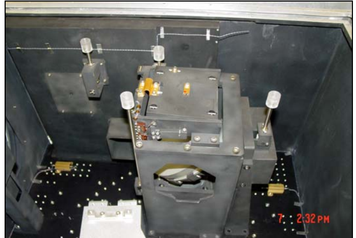
14. Upper Grating remove 6 mounting screws and slide unit up to separate from lower sections.
